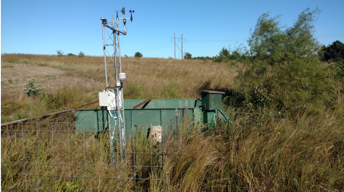
Figure 4: Watershed outlet with weather station, H-flume and stilling well attachment, Shaft Encoder, ISCO 3700C Autosampler, and stratus precision manual rain gauge equipment. Manual rain gauge was not visible due to herbaceous vegetation and shaft encoder was also not visible due to protective wooden green box cover. Photo was taken near Prairie to Switchgrass (P-SG) watershed within the Cross Timbers Experimental Range near Stillwater, OK, USA.
