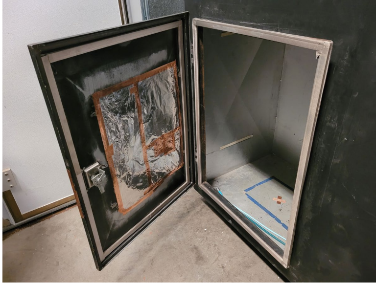
Figure A.6.: New gaskets on the perimeter of the enclosure’s door frame and door. Aluminum foil has been added over the back side of the window to prevent anymore leakage out of the left window.
