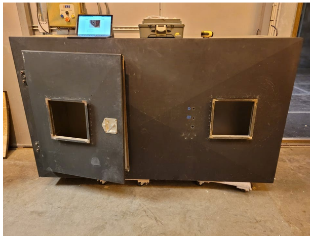
Figure A.1: Small chamber without windows sealed (pre-repairs)
