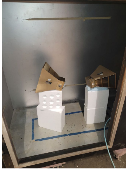
Figure A.12.: Antenna placement and orientation for the small chamber's AD test.
