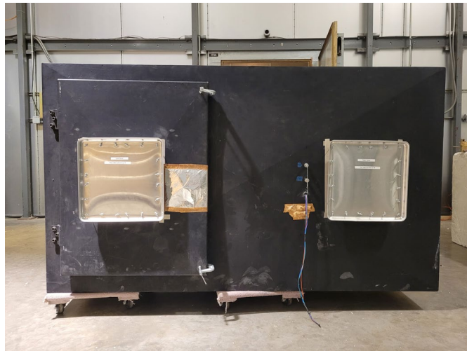
Figure A.5.: Small chamber post repairs with aluminum panels covering both windows. The door handle was covered because it was leaking energy at its seams. The use of two clamps were used to keep the door tightly shut. (post repairs)
