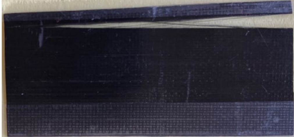
Figure 21: Composite Coupon that was separated from group of tows. Signs of fiber tearing occurring from the separation
