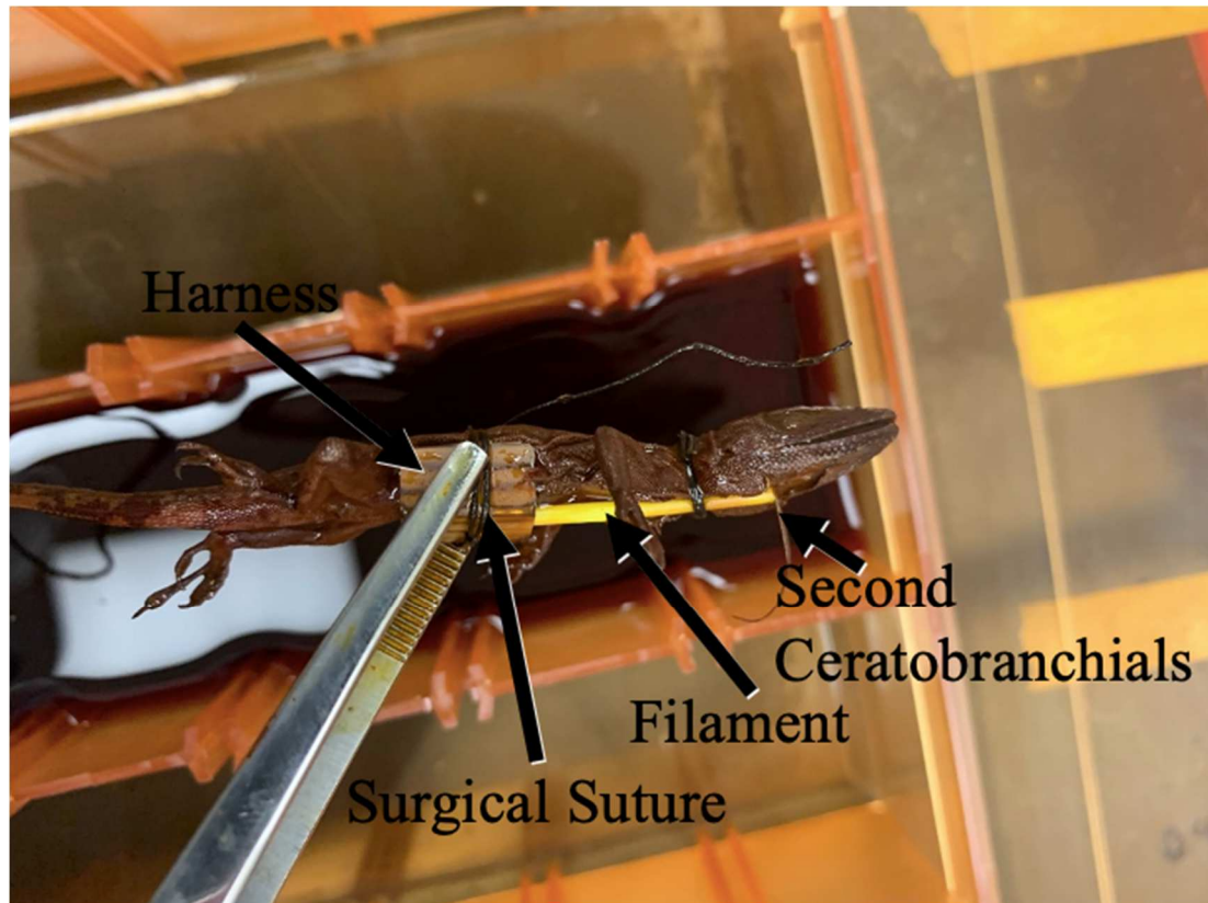
Figure 2.3. Representation of brace harness on specimen. Specimen undergoing diceCT staining process with hyoid bones extended. Observable here are the printed harness (brown), the 3D printer filament (yellow), and surgical suture (black). Projected second ceratobranchials can be observed against the right tip of the 3D printed filament.
