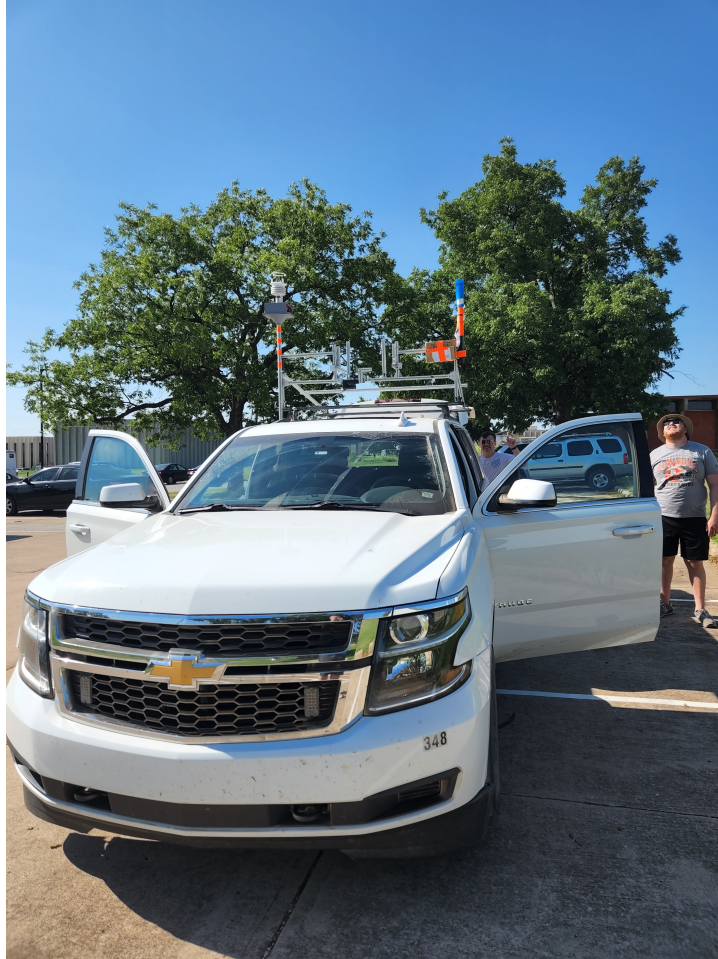
Figure 57: Vehicle Setup to Simulate Mobile Mesonet
