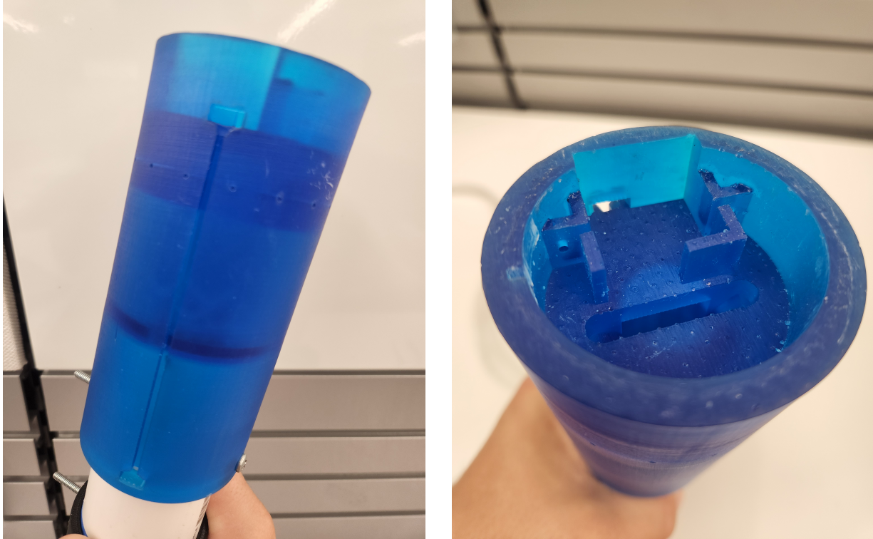
Figure 31: Cylindrical Multi-hole Probe's Internal Compartment.
