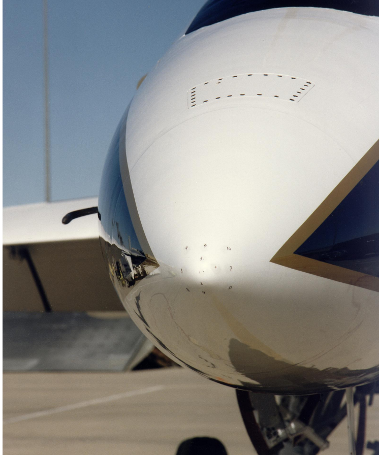
Figure 12: FADS system on the nose of NASA's F/A-18 Systems Research Aircraft[7]
