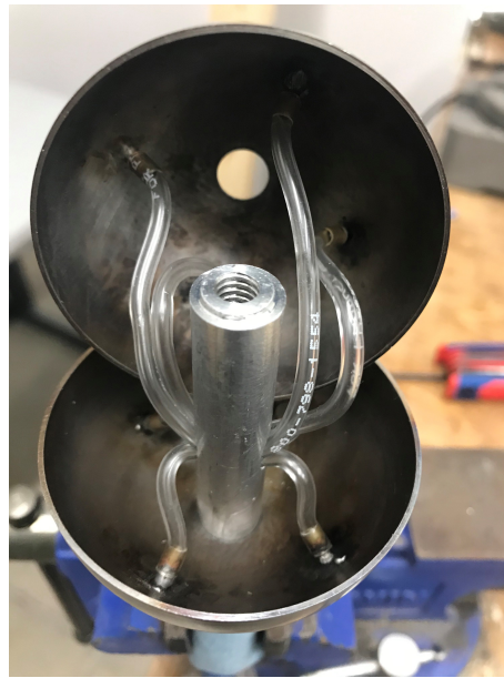
Figure 29: Spherical Probe Internals
