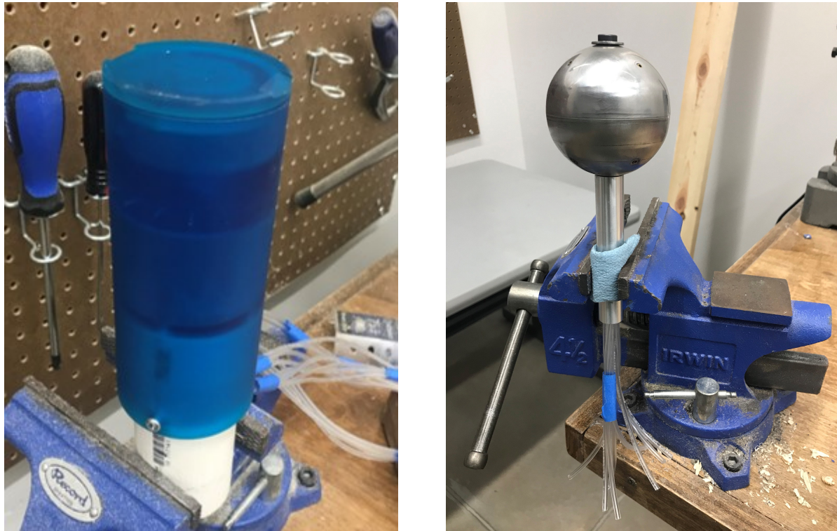
Figure 28: Cylindrical and Spherical Probe Designs.
