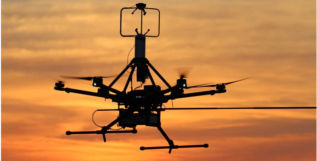
Figure 24: DJI Matrice 600 outfitted with a Young 8100 and aerosol sensor[4]
