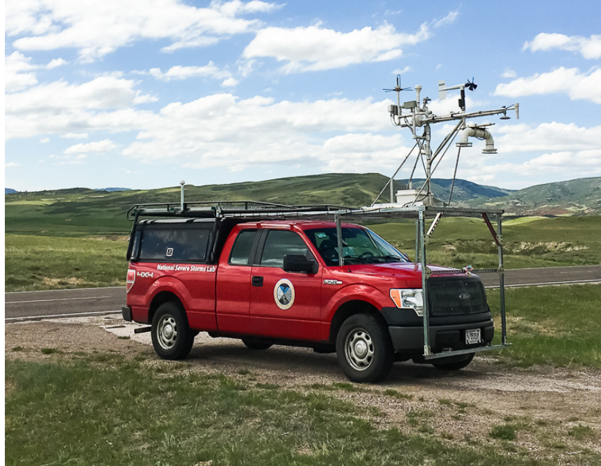
Figure 22: Mobile Mesonet used by the National Severe Storm Laboratory[21]
