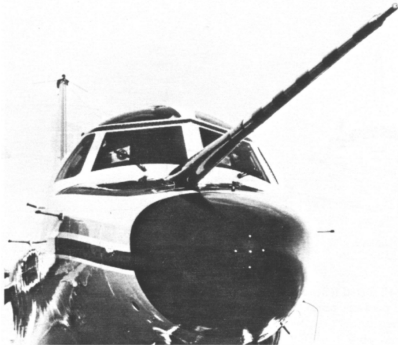
Figure 23: A Multihole Probe Equiped on a NCAR C130Q Hercules[14]
