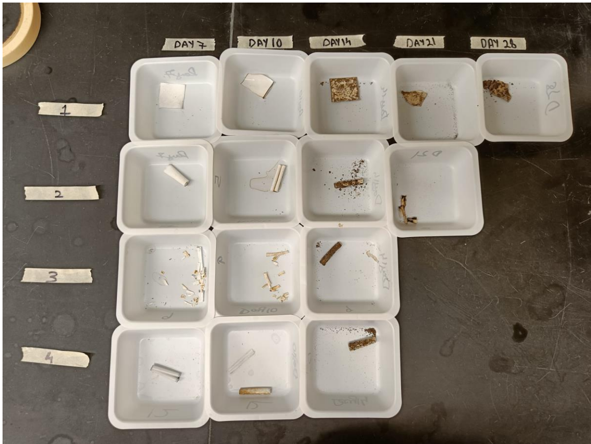
Figure 4.1: PLA sampled on days 7, 10, 14, 21 and 28. The four different treatments included 1) Control, 2) Autoclaved Plastic composted in control, 3) Autoclaved plastic with compost starter, 4) Heat treated plastic with compost starter
