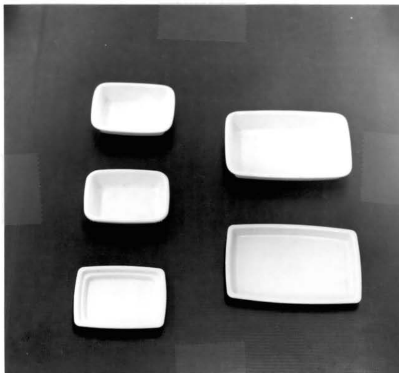
Fig. 5.5 Five Different Rectangularly Shaped Ceramic and Plastic Dishes Top to Bottom, Left to Right: Small Plastic Dish, Small Ceramic Dish, Small Plastic Spacer, Large Ceramic Dish, Large Plastic Spacer
