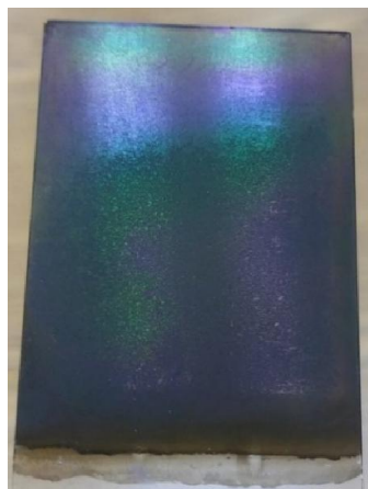
Figure S5: Interference of visible light on a nickel oxide (NiO) film. The film was prepared by pyrolysis of a nickel acetate hydroxide film.
