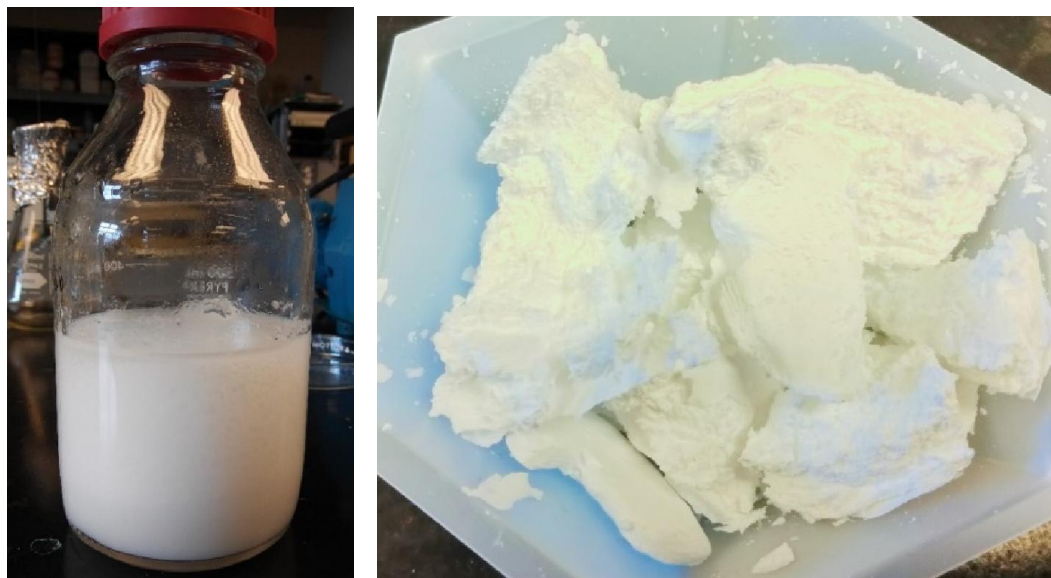
Figure 3: Hydrolysis reaction of zinc acetate and propylene oxide in water at 40°C (left) and its dried product zinc acetate hydroxide, \text{Zn}(\text{OAc})_{0.33}(\text{OH})_{1.67} \cdot 0.50\text{H}_2\text{O} (right)
