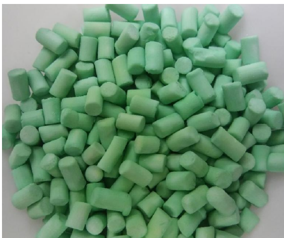
Figure 13: Nickel acetate hydroxide decorated silica pellets, prepared by hydrolysis of nickel acetate aqueous solution and silica pellets.
