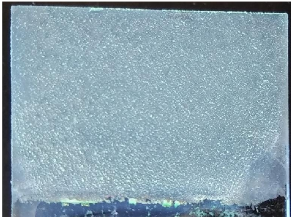
Figure 2: \beta -Ni(OH) 2 film grown on a microscope glass substrate from saturated nickel hydroxide-aqueous ammonia solution.
