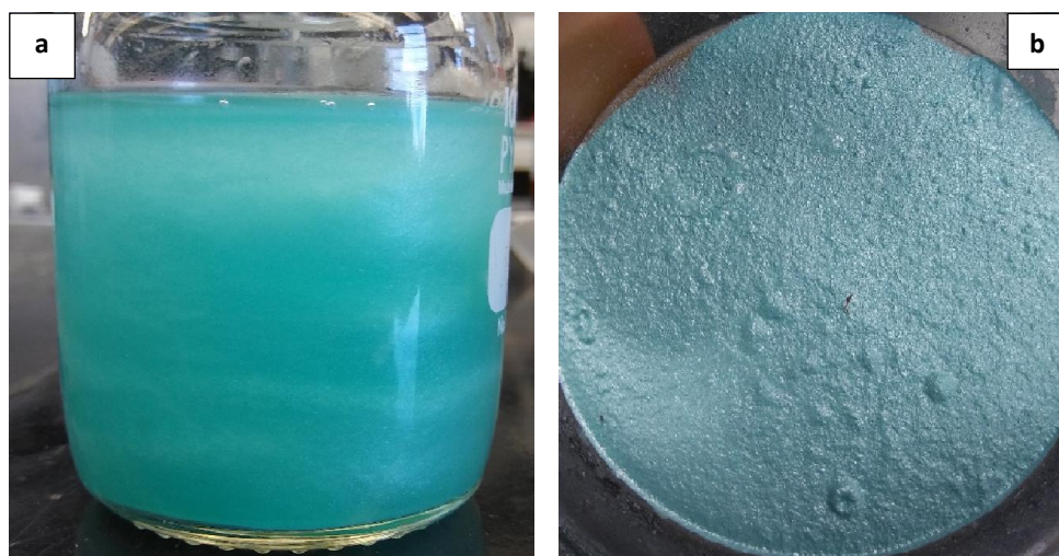
Figure 2: Bluish-green crystalline copper acetate hydroxide, \text{Cu}(\text{OAc})_{0.44}(\text{OH})_{1.56} \cdot 0.50\text{H}_2\text{O} synthesized at 40°C. (a) The crystalline product in water during washing, exhibiting diffraction of visible light, and (b) isolated product.
