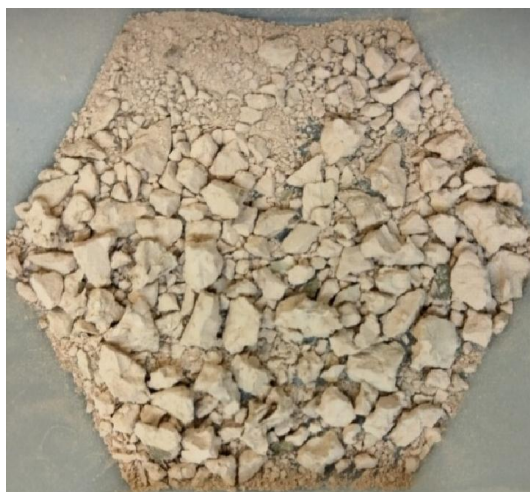
Figure 5: Nickel-cobalt hydroxide, \text{NiCo}_2(\text{OAc})_{0.05}(\text{OH})_{1.95} \cdot 0.4\text{H}_2\text{O} prepared from hydrolysis of aqueous 2:1 cobalt acetate and nickel acetate with propylene oxide.
