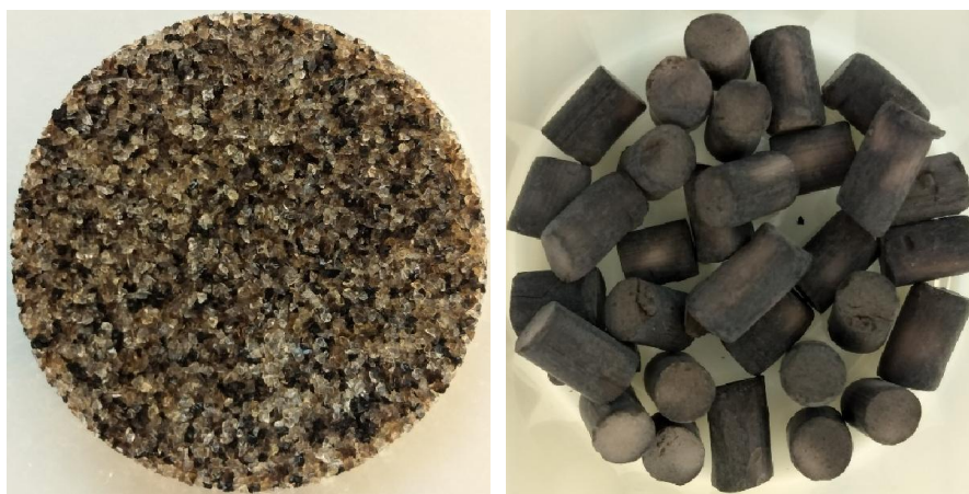
Figure 7: Cobalt oxide, \text{Co}_3\text{O}_4 decorated silica-gel (left), and silica-pellets (right) prepared by pyrolysis of \text{Co}(\text{OH})_2 deposited silica-gel and silica-pellets at 600 °C.
