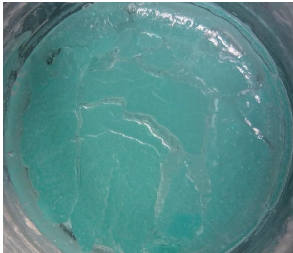
Figure 3: Aluminum substituted \alpha -nickel hydroxide membrane grown from saturated hexamine nickel(II) hydroxide and sodium aluminate solution.
