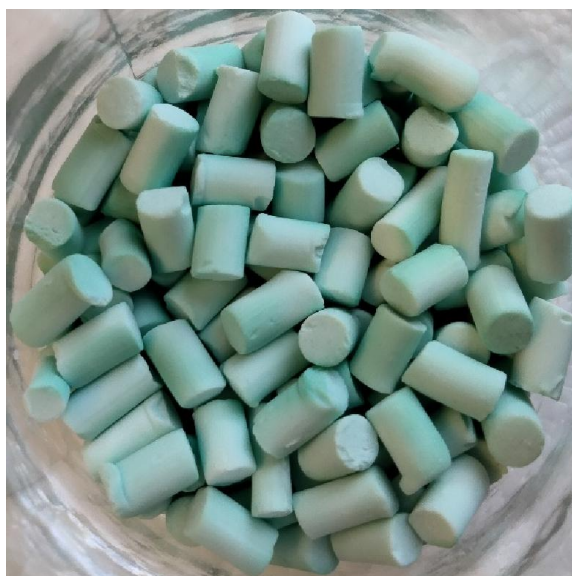
Figure 21: Nickel-copper acetate hydroxide, \text{Ni}_{0.55}\text{Cu}_{0.45}(\text{OAc})_{0.30}(\text{OH})_{1.70}\cdot n\text{H}_2\text{O} deposited silica pellets
