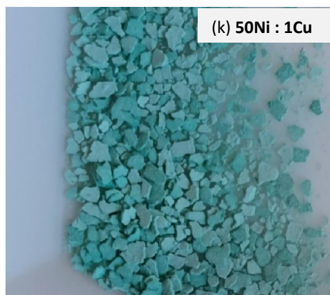
Figure S1: Camera pictures of the products of hydrolysis of nickel acetate and copper acetate mixtures at various ratios – (a) 1Ni : 9Cu, (b) 1Ni : 3Cu, (c) 1Ni : 2Cu, (d) 1Ni : 1Ni, (e) 2Ni : 1Cu, (f) 3Ni : 1Cu, (g) 4Ni : 1Cu, (h) 6Ni : 1Cu, (i) 7Ni : 1Cu, (j) 9Ni : 1Cu, and (k) 50Ni : 1Cu.
