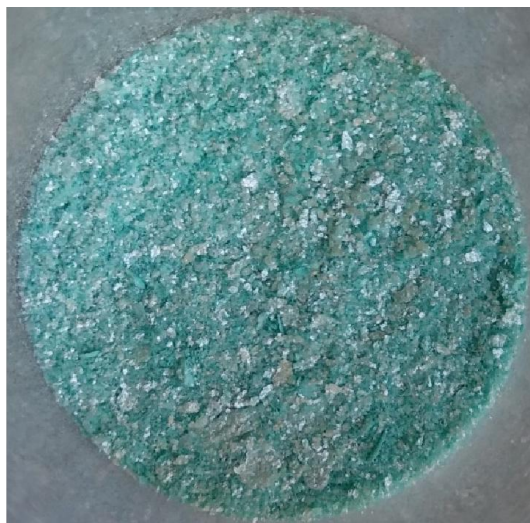
Figure 1: Copper acetate hydroxide, \text{Cu}(\text{OAc})_{0.44}(\text{OH})_{1.56} \cdot 0.40\text{H}_2\text{O} synthesized at 60 °C.
