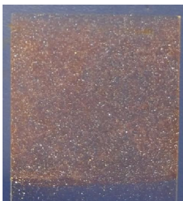
Figure 4: \text{Cu}_2\text{O}/\text{CuO} decorated glass substrates prepared by hydrolysis of 0.49 M aqueous solution of copper formate at 90 °C for 48 hours.
