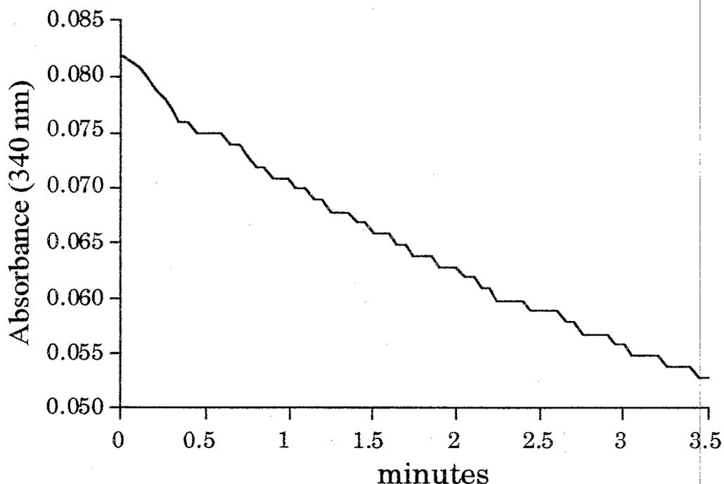
Figure 1. FAS Assay Linearity over Time. The linearity of decrease in absorbance at 340 nm. The reaction was in pH 7.4 buffer, 100 mM NADPH, 60 mM acetyl-CoA, 400  $\mu$ l final volume. The reaction was started by adding 10  $\mu$ l of 2.4 mM malonyl-CoA (60  $\mu$ M final concentration) and the absorbance was measured at 3 second intervals.
