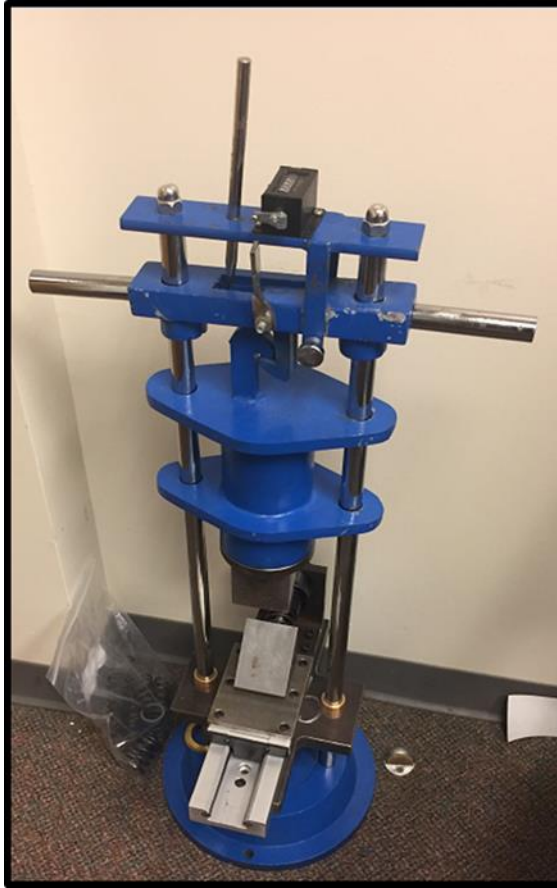
Figure 2.3 Complete assembly of the impact tester used to simulate automotive paint smears.
