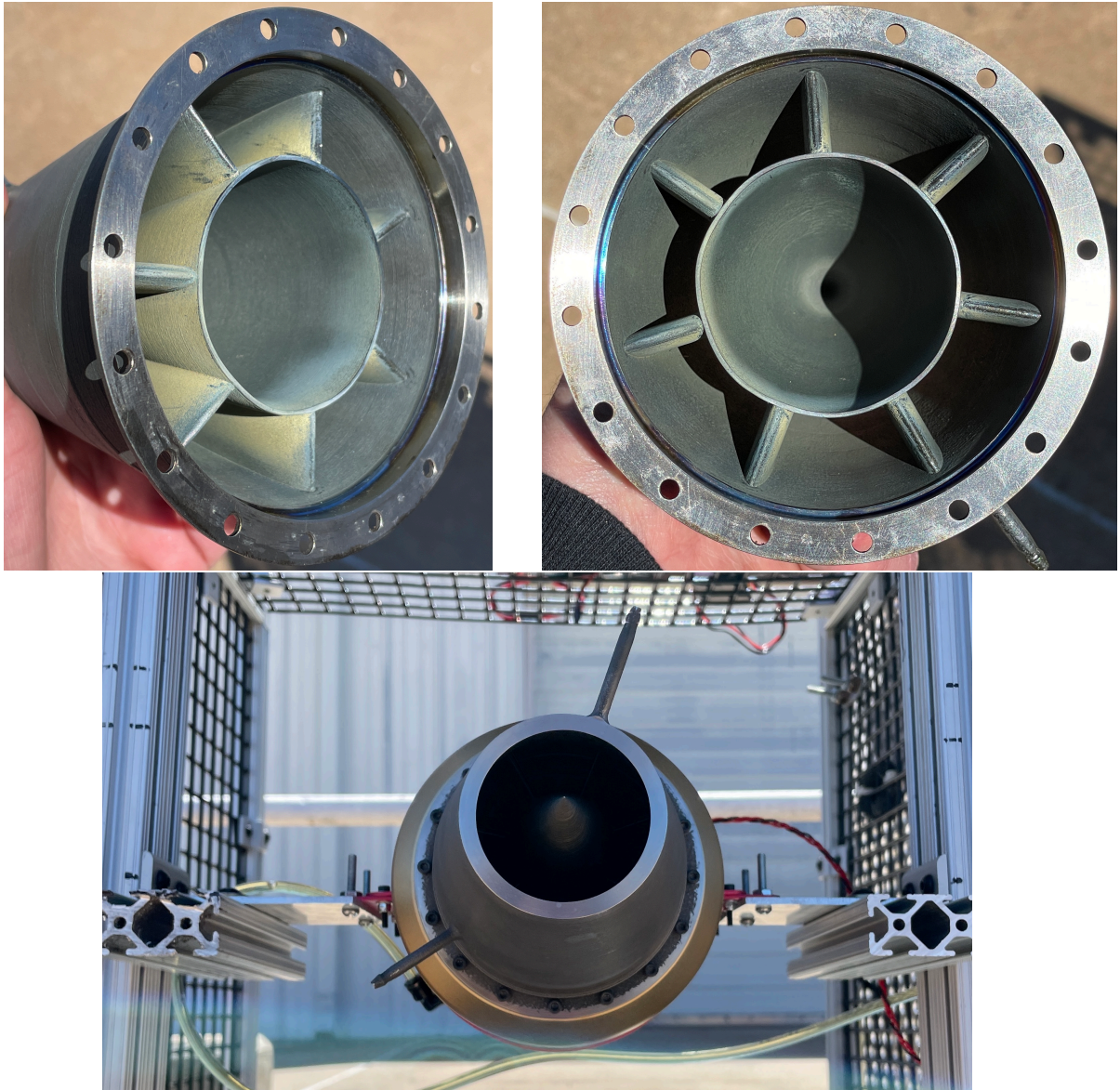
Figure 36: Exit area for the thermal nozzle likely too small for the K320
