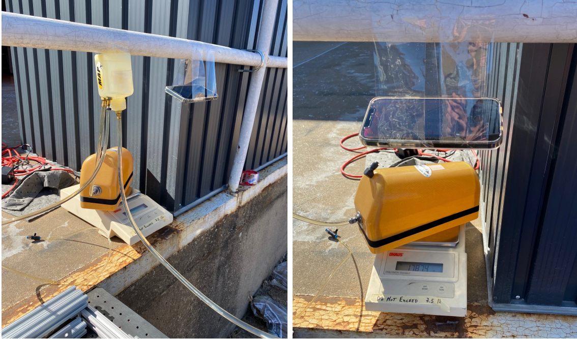
Figure 27: Experimental setup for measuring mass flow rate of fuel.
