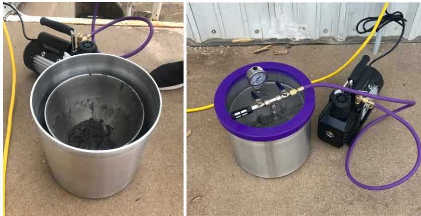
Figure 11: Propellant Degassing Chamber Configuration
