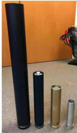
Figure 3: 76mm (Left), 54mm (Middle) & 38mm (Right) Rocket Casings
