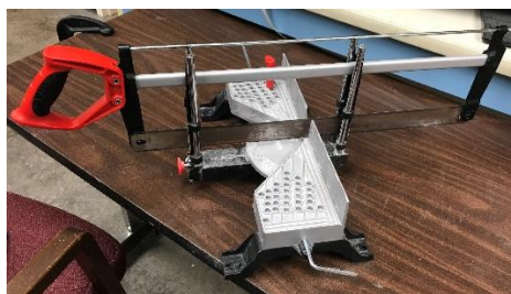
Figure 13: Adjustable Mitre Saw for Cutting Propellant Grains
