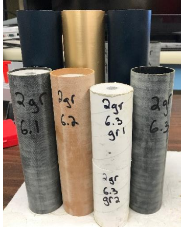
Figure 14: Liner, Propellant Grain, and Casing Fit Checking
