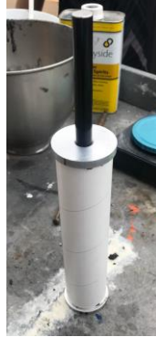
Figure 12: Casting of 54 mm Motor with Aluminum Casting Caps and Coring Rod
