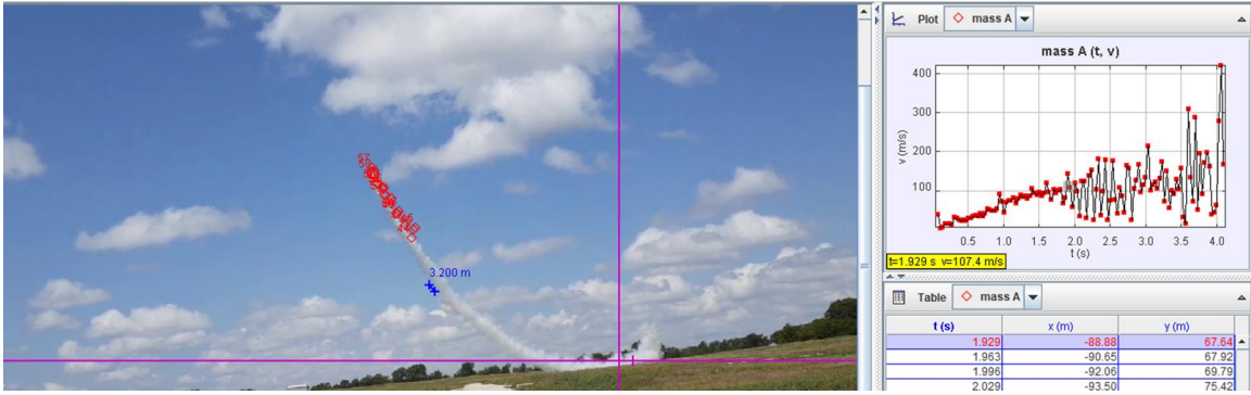
Figure 34: Video Analysis of Previous Launch using Tracker Software
