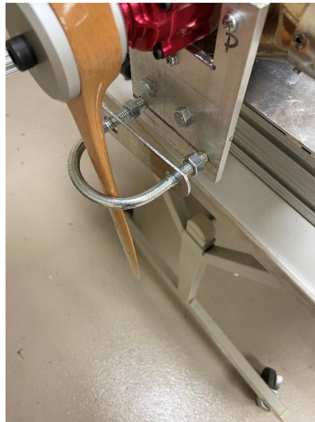
Figure 33: U-bolt Propeller Lock (missing padding)
