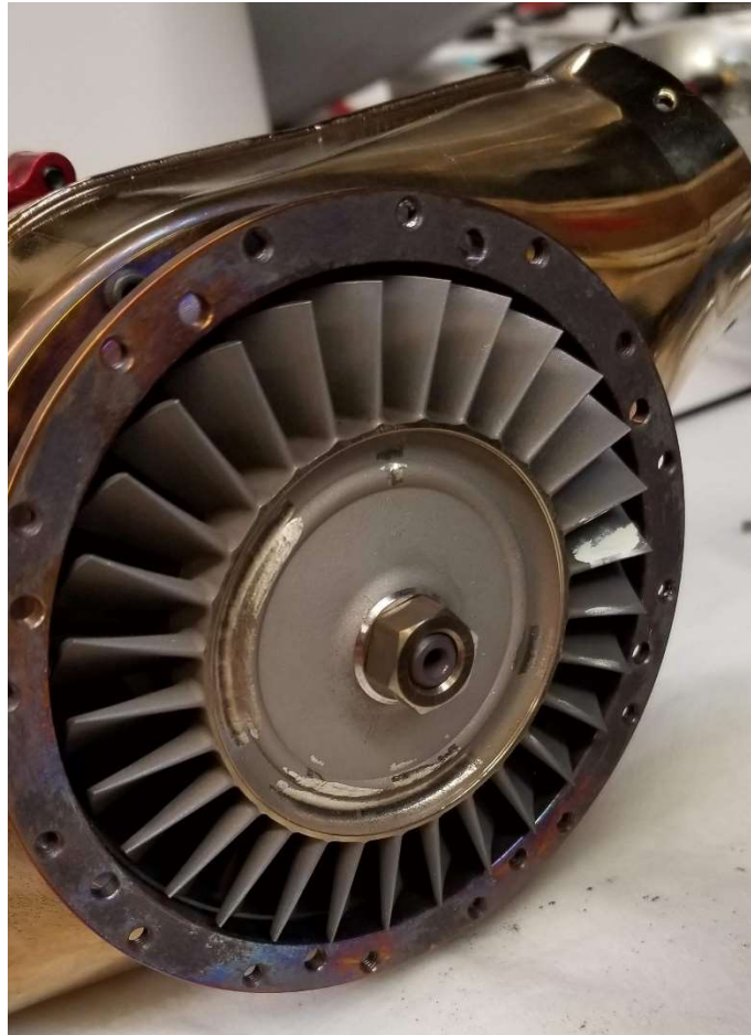
Figure 7. A photo of the Kingtech K-100TP secondary turbine. Additionally, the exhaust manifold can be seen behind the turbine.
