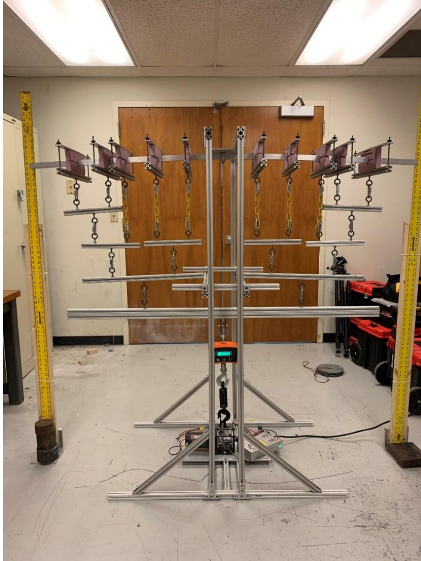
Figure 76: Aluminum Beam Yield Experiment
