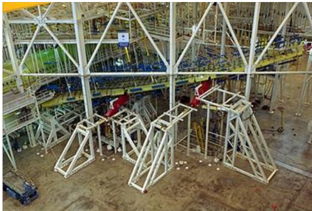
Figure 15: Airbus A-380 Static Wing Test
