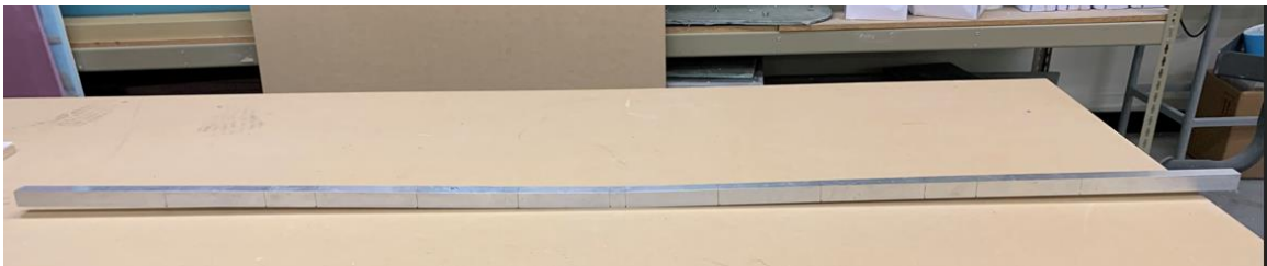
Figure 77: Permanently Deformed Aluminum Beam
