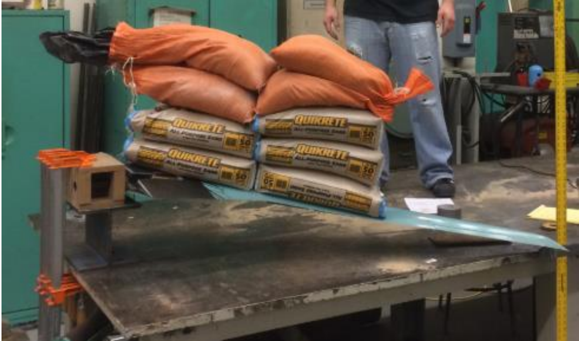
Figure 7: Sandbag Test Of Cessna Citation Longitude Wing
