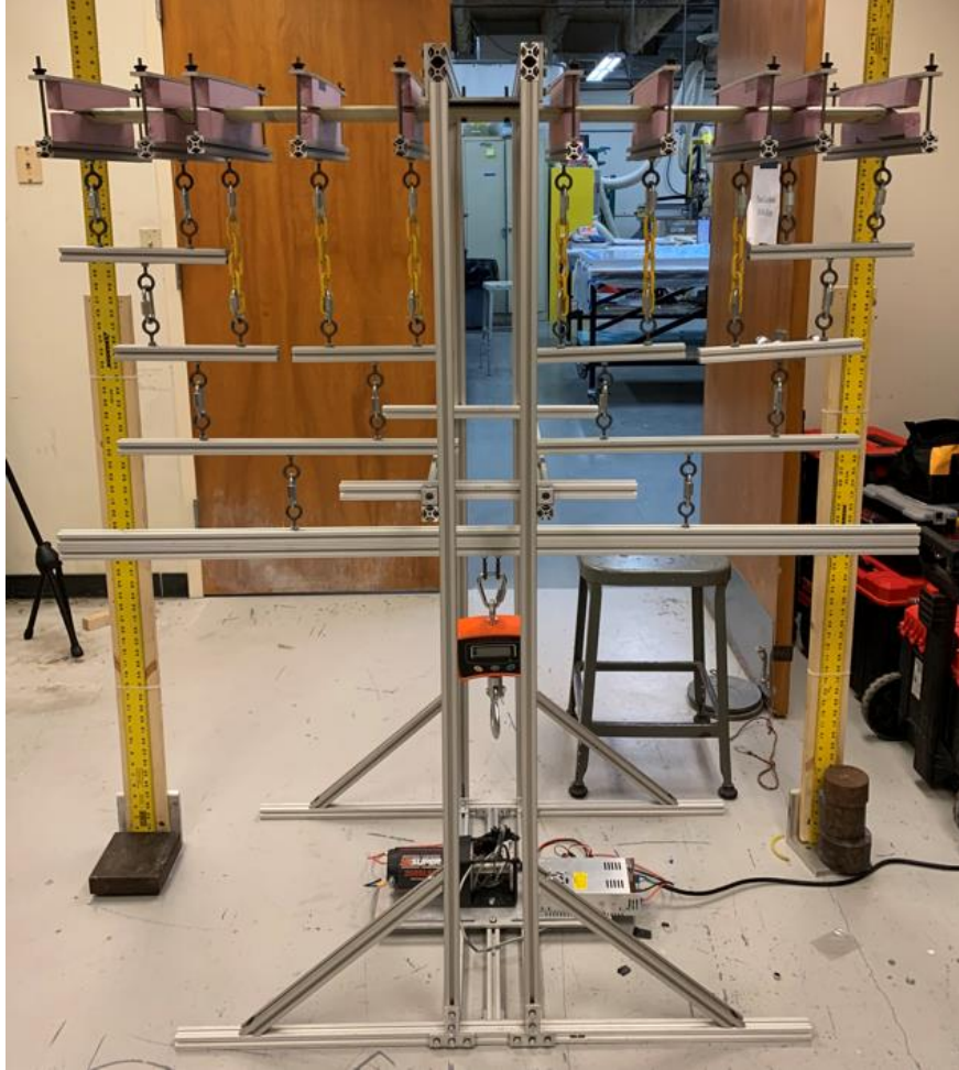
Figure 78: Composite Wing Setup Before Testing
