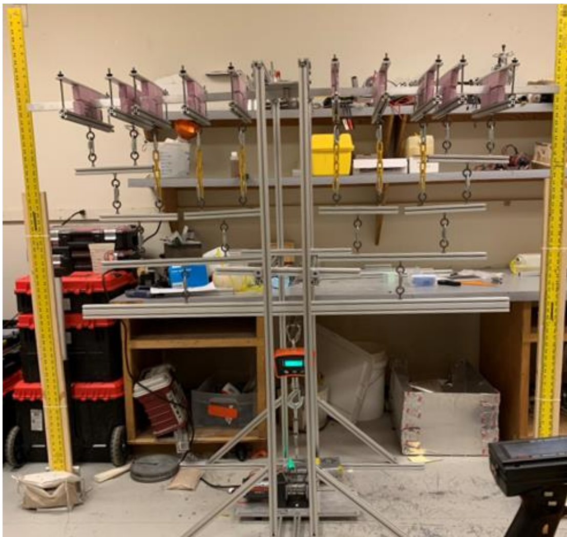
Figure 74: Aluminum Beam Deflection Experiment
