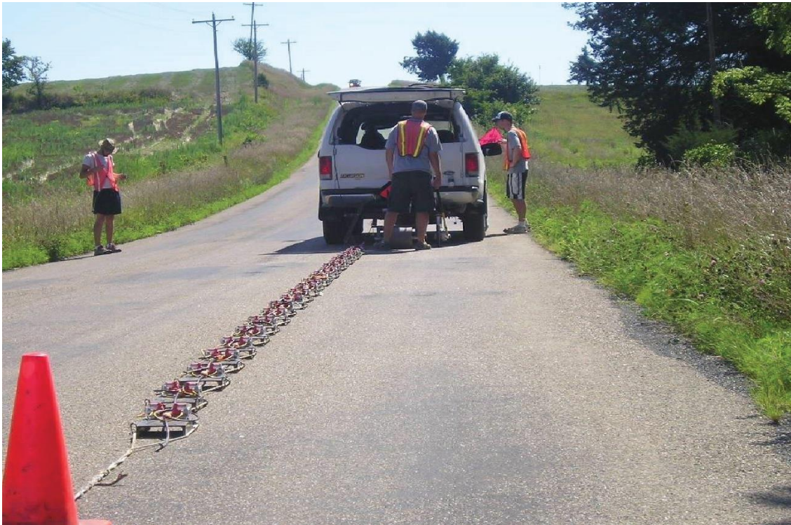
Figure 2.4. SH-wave seismic data acquisition utilizing the land streamer system at McHenry County, northern Illinois.
