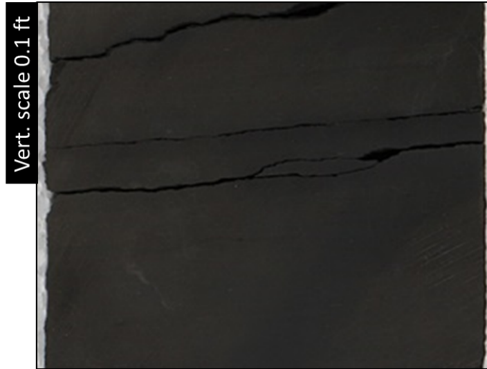
Figure 20: Close up core photograph of facies F6; massive muddy turbidite in an argillaceous mudstone.
