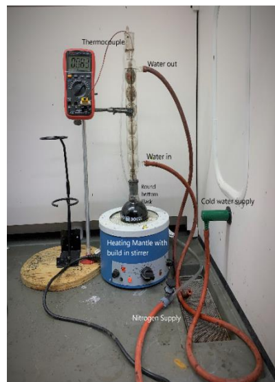
Fig. 2.1: Schematic representation (left) and lab set-up (right) of redox reaction reactor set up.
