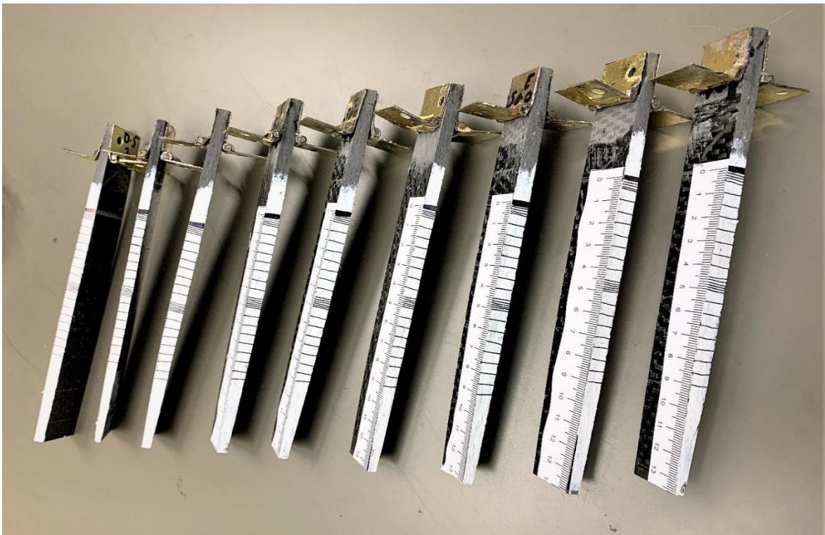
Fig. 3.5: Ready to test DCB samples.
