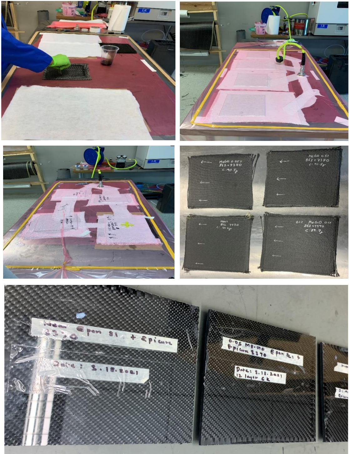
Fig 3.2: CFRP samples and preparation process
