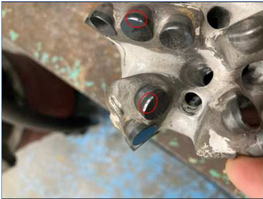
Figure 4.13. Artificially Worn PDC Bit
