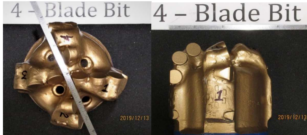
Figure 3.2. Profile of the 4-Bladed PDC Bit Design
