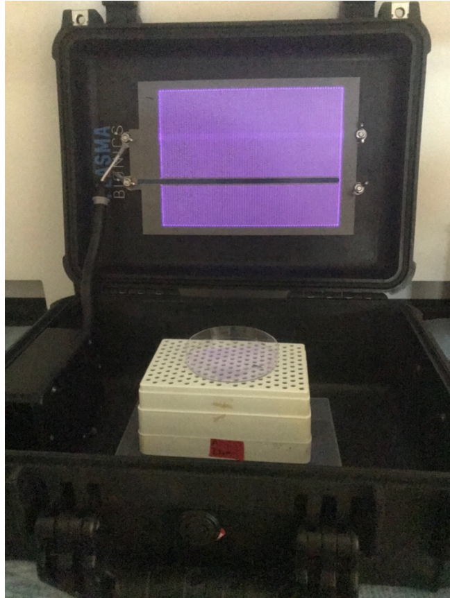
Figure 1: Picture of ACP Device 1.0 with actuator A1 operating at an uniform full glow. The actuator was attached via wing nuts, which allowed the switching of actuators. The lid was closed and latched to ensure a close system when the treatment was performed.
