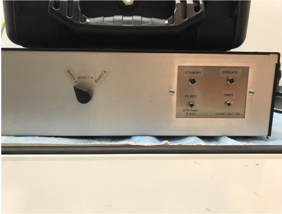
Figure 10: The added switches & knobs on the power supply of ACP Device 3.0
