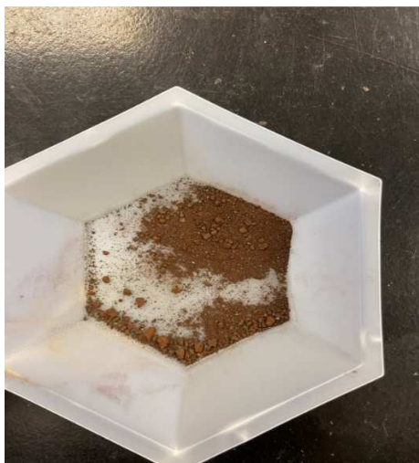
Figure 4-10 product of precipitation reaction as iron hydroxide
