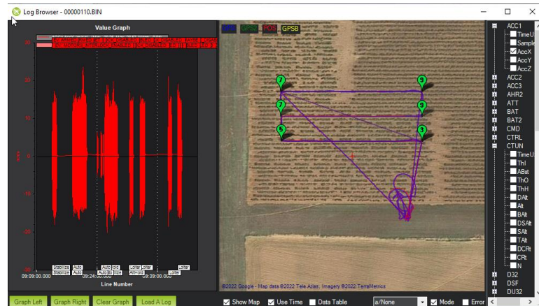
Figure 6. Mission Planner Dataflash Log Analyzer
