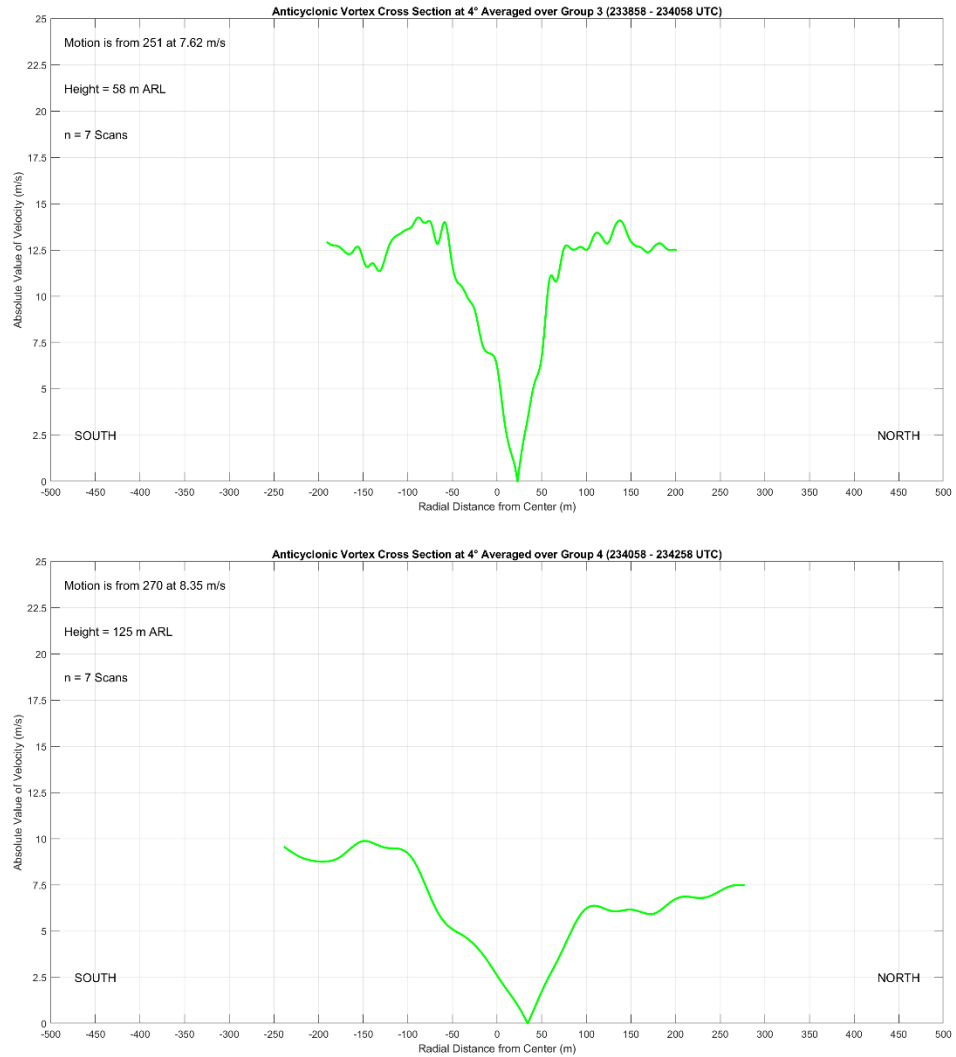
Figure 7.12: Azimuthal Cross Sections through the Selden anticyclonic Tornado at 4° elevation for track segments 3 (top) and 4 (bottom).
