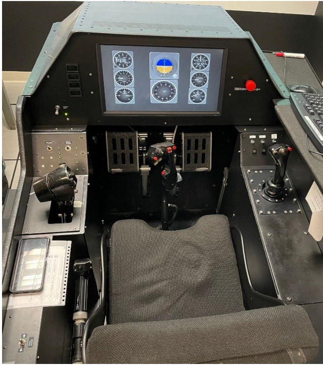
Figure 1. Simulator Pilot Seat, Controls, and Primary Flight Display.
