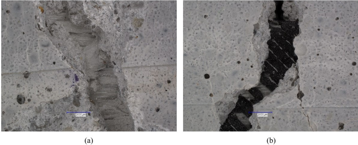
Figure 65: Microscopic images of PolC reinforced with (a) VAHT unidirectional GFRP (b) 3D printed unidirectional GFRP
