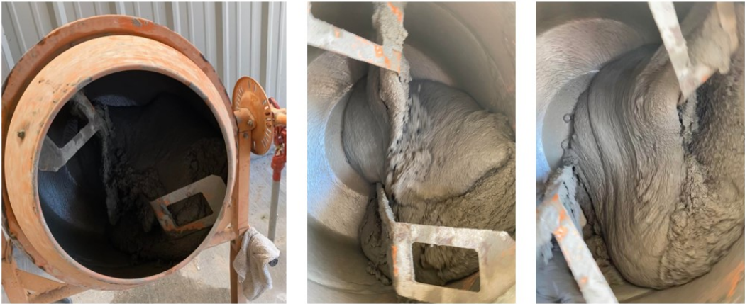
Figure 19: Portland cement concrete mixing process
