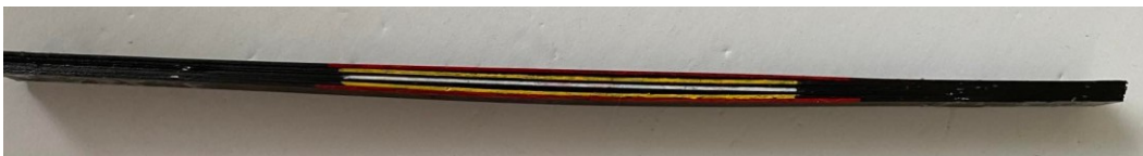
Figure 15 : 3D printed multidirectional coupon GFRP (High Strength)
