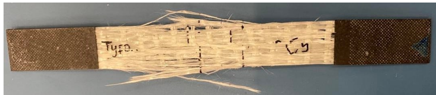
Figure 31: Failed VAHT unidirectional GFRP
