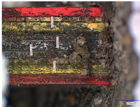
Figure 67: Microscopic image of PCC reinforced with Multidirectional 3D printed GFRP
