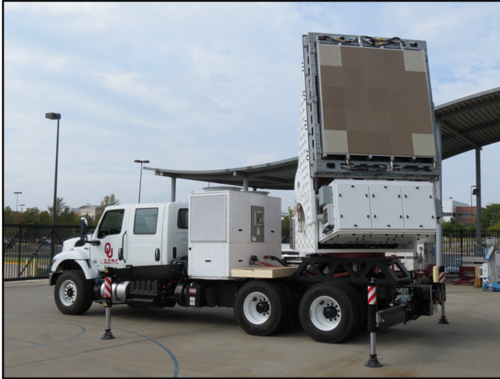
Figure 3.7: The mobile Horus is an S-Band, dual-polarization, fully digital radar [71].
