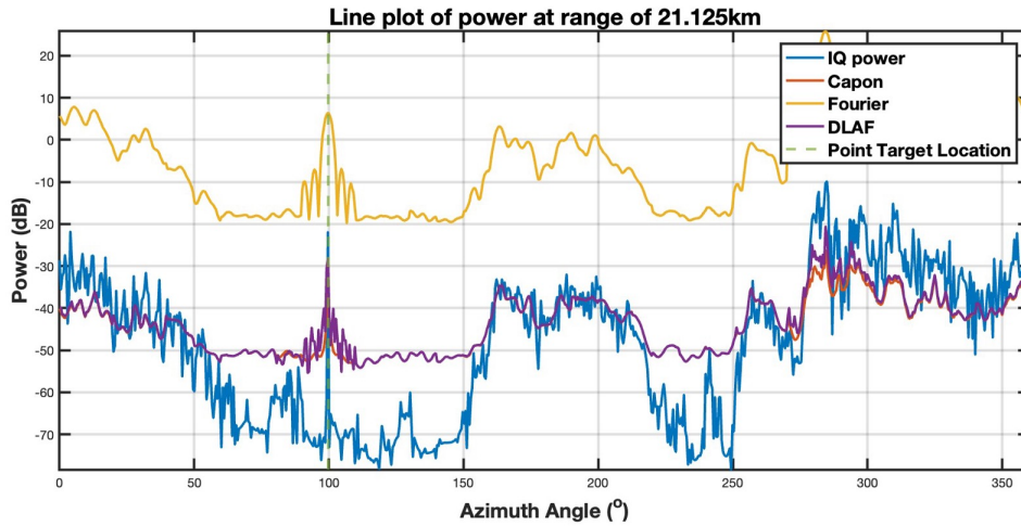
Figure 5.8: Power (dB) by the Capon, the Fourier, and DLAF methods at the range 21.125km for 360° in azimuth of the supercell case.
