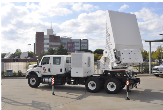
Figure 3.6: A picture of C-band mobile Polarimetric Atmospheric Imaging Radar (PAIR) is shown.
