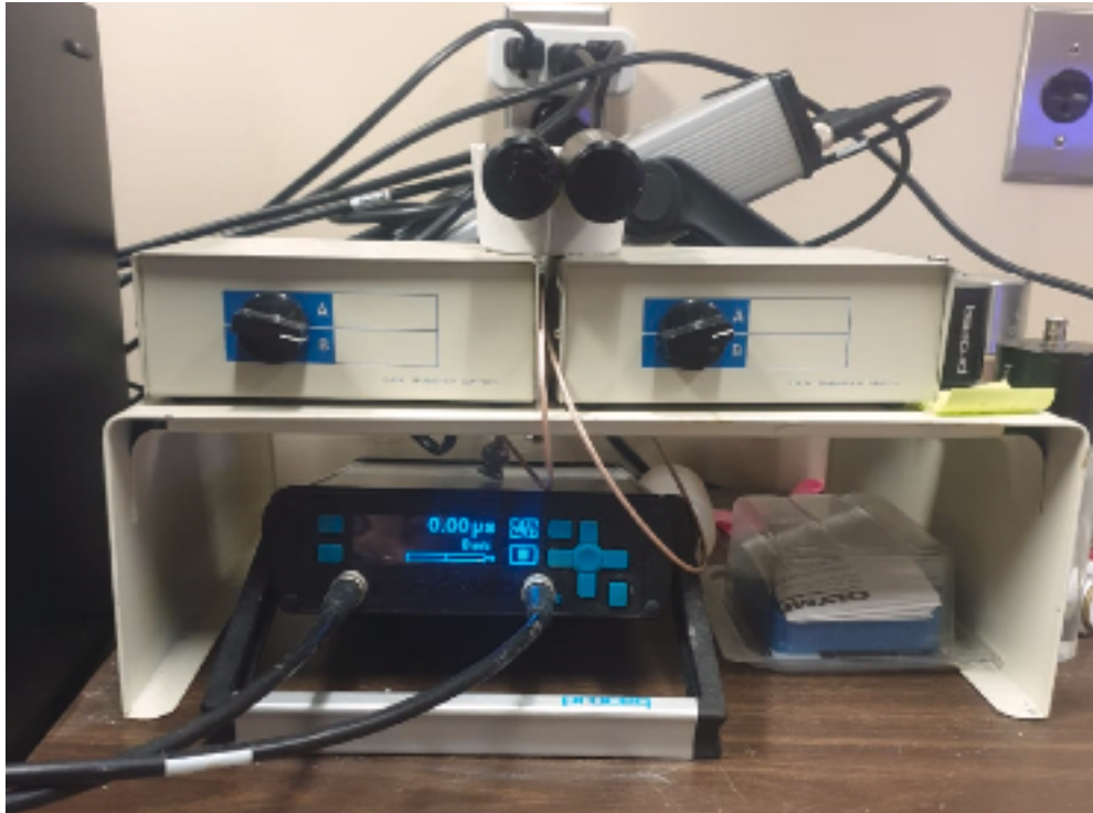
Figure 10.-Proceq™ Ultrasonic Device for the UPV test.
