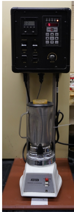
Figure 7.-Ofite-20 cement mixer used for the mixing process.
