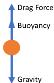
Figure 2-7 : Force balance on a liquid droplet
