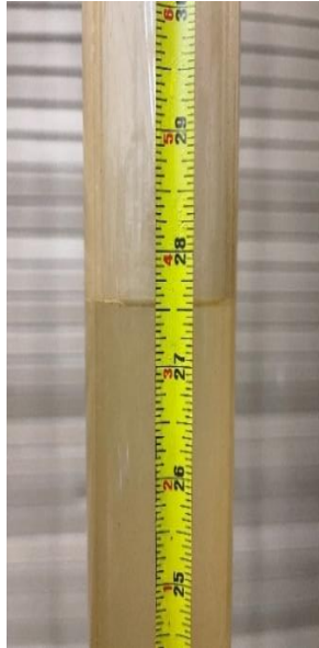
Figure 3-12: Liquid level for a test at v_{SL} = 0.0033 \text{ m/s} and v_{Sg} = 9.15 \text{ m/s}
