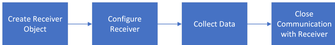
Figure 3.2. Hotstart Script Operations: When Hot Start is enabled, the script creates a Receiver of a child class as defined in the configuration, configures the GPS receiver according to the implementation in the given child class, collects the data, and stops communication with the receiver so that it may be used for other processes later in the program.
