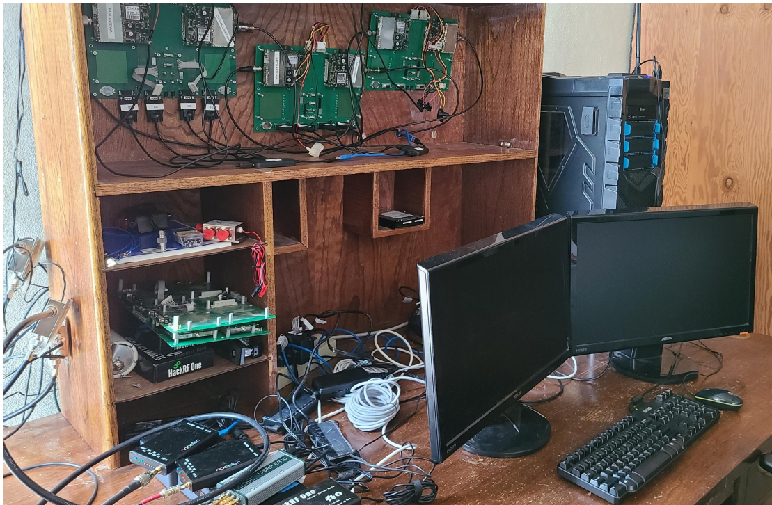
Figure C.7: GBAS Ground Base Station setup. Mounted on the back wall are the GG12s connected to the GBAS PC via multiple serial to USB cables. The SDRs are connected to their respective Intel NUCs at the lower left which are connected via a network switch to the GBAS PC.
