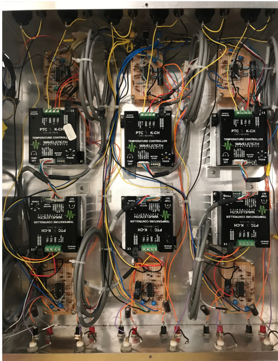
Figure 4.15: A homemade current controller for the bias coil. There are six individual channels that can output a current range from -5\text{ A} to 5\text{ A} . Each of them uses a commercial ultra-low noise TC (Wavelength Electronics PTC5K-CH) as a current controller. An extra external setpoint circuit and a sensing circuit are used to convert the signal to a readable signal for the TC.
