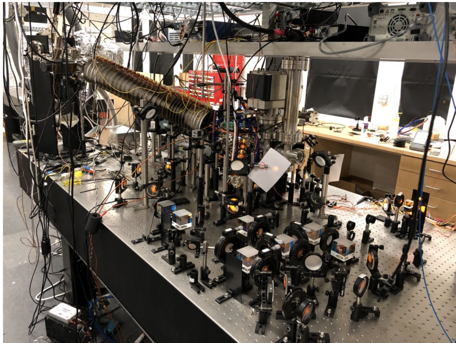
Figure 4.11: The 4' \times 10' non-magnetic optical table that holds the MOT optical system, and the vacuum system. The laser beams generated on the main laser table are delivered to this table via PM fibers to generate the MOT.
