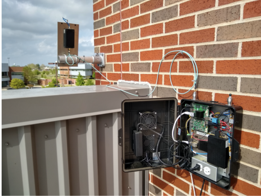
Figure 2.6: Picture of a bistatic receiver from Byrd et al. (2019). This specific system is mounted on the roof of the Radar Innovation Laboratory at the University of Oklahoma in Norman, Oklahoma.
