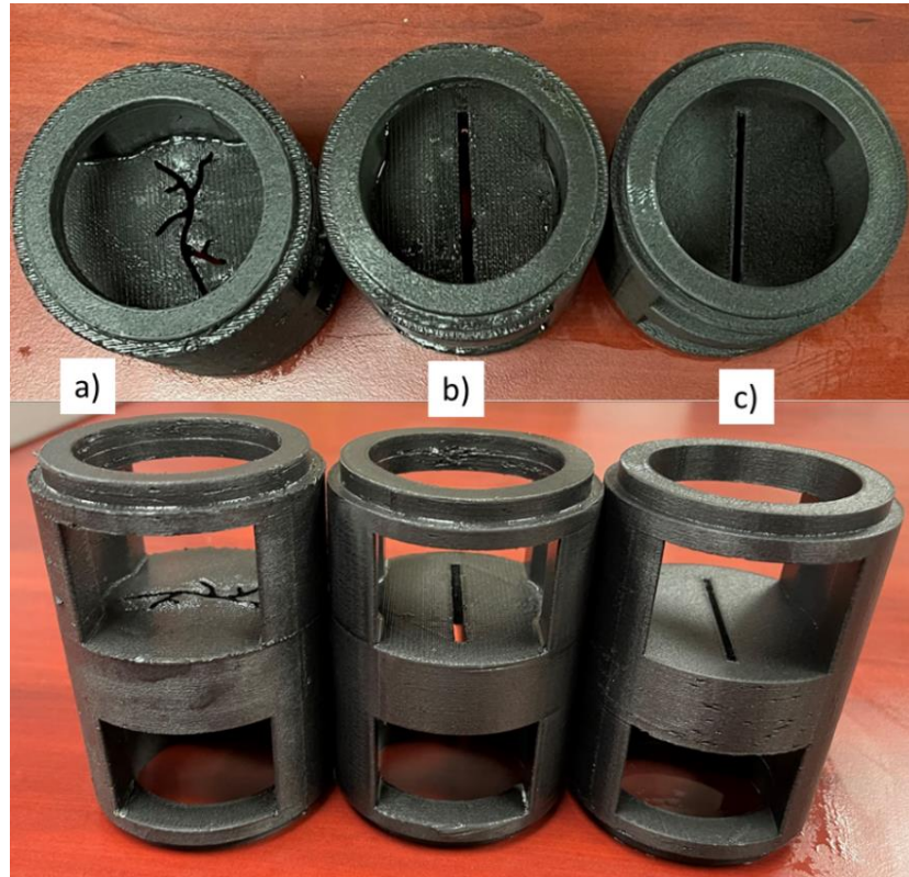
Figure 4.6: 3D fractured discs used in this study: a) complex fracture, b) 3000 microns, and c) 2000 microns.
