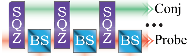
Figure 5.11: Model for squeezing generated in an absorptive medium. The squeezing operator is broken up into an infinite number of infinitesimal parts composed of a stage of loss in the probe from beam splitters after each stage of squeezing.
