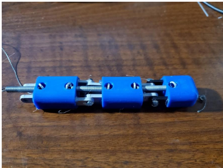
Figure 26 3D printed finger assembled
