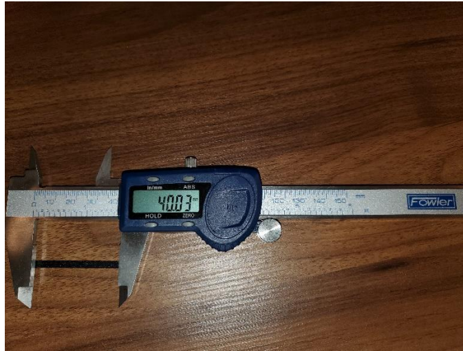
Figure 35 40x3x2 mm test sample
