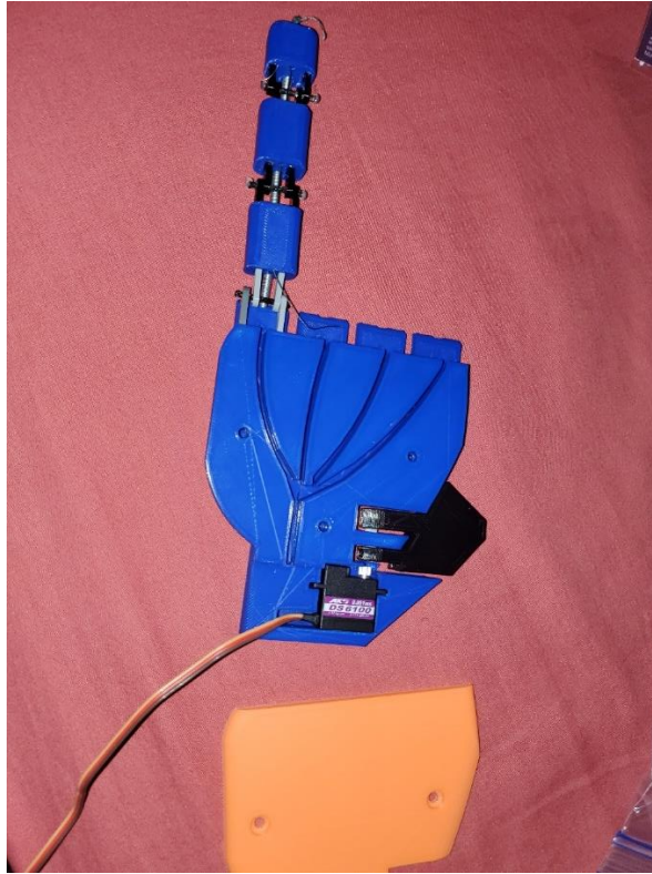
Figure 27 3D printed, palm and finger assembled with motor installed
