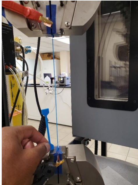
Figure 48 TPU 95A test sample and setup
