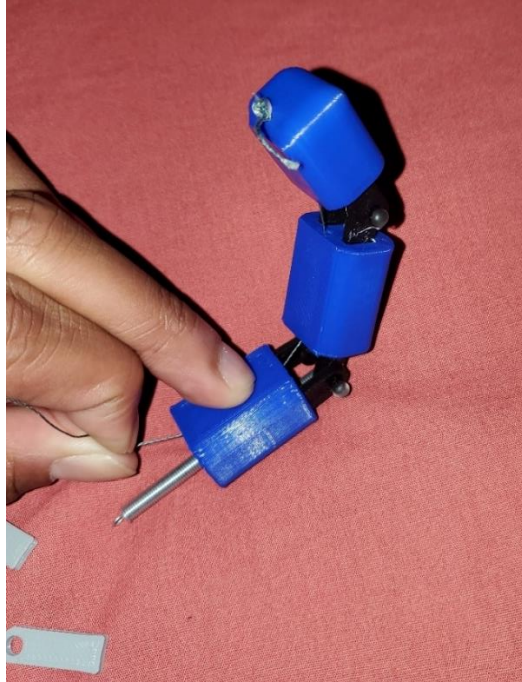
Figure 28 3D printed finger bent
