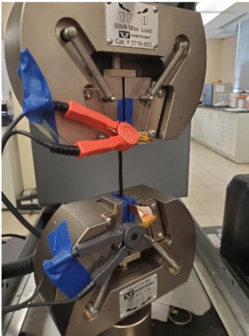
Figure 50 CPLA test sample and setup
