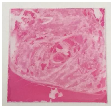
Figure 4.1 Image of an amorphous \text{TiO}_2 thin film loaded following \text{SiO}_2 thin film loading protocol
