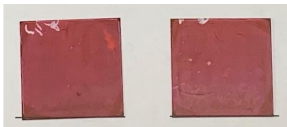
Figure 4.30 Film duplicates kinetically doped in 4mM dye loading solution of 1 mM each R6G, AO, Ru2, and Nile blue in 10 mM phosphate buffer at 0-minute post spin-coat delay
