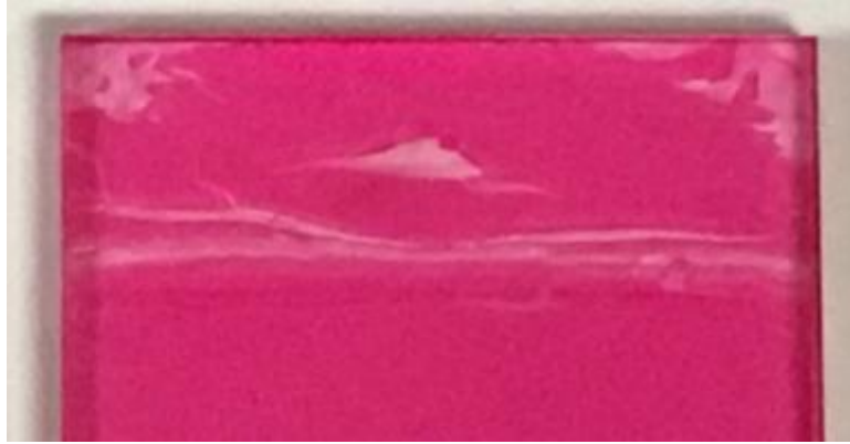
Figure 4.3 Example break in thin film caused by an extended moment of liquid-air interface
