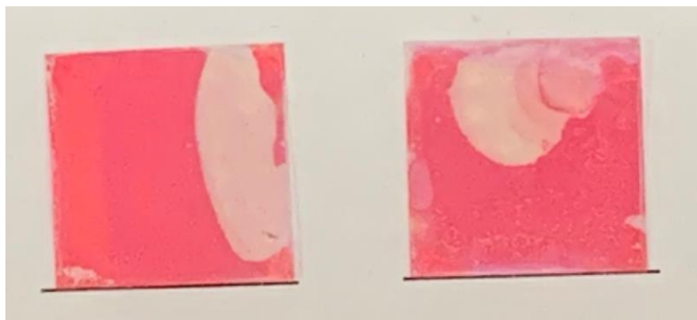
Figure 5.2 Examples of leaching damage caused by standing water during hydrothermal annealing
