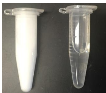
Figure 3.1 A comparison of sol-gel solutions when reagents are added in the incorrect(left) or correct (right) order.
