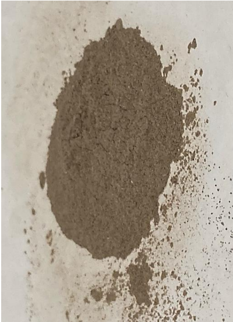
Figure 12. Diatomaceous earth before placed into the central zone.
