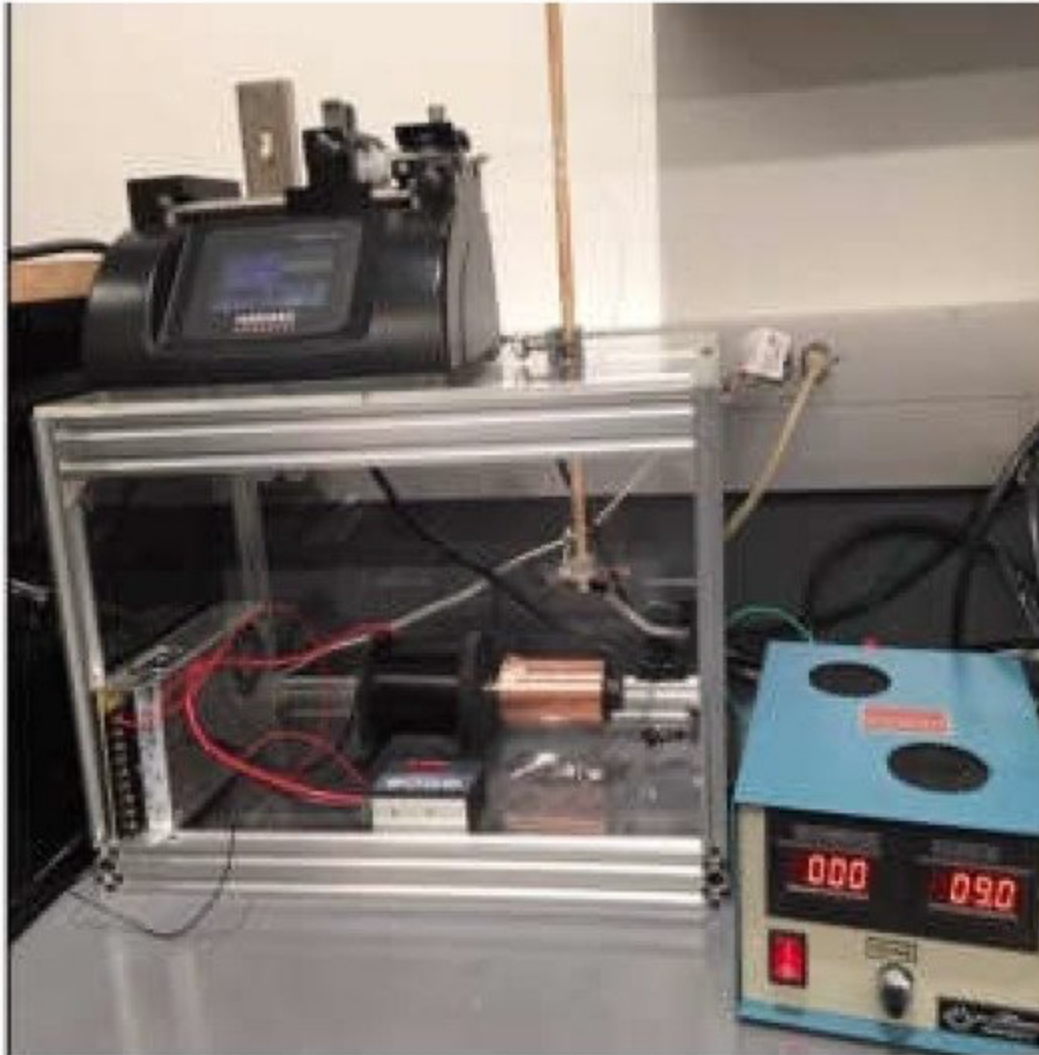
Figure 8. Electrospun fabrication unit used to produce the nanofiber dressing.
