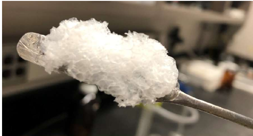
Figure 6.6. MSA particle shell remains after foam trial completion.
