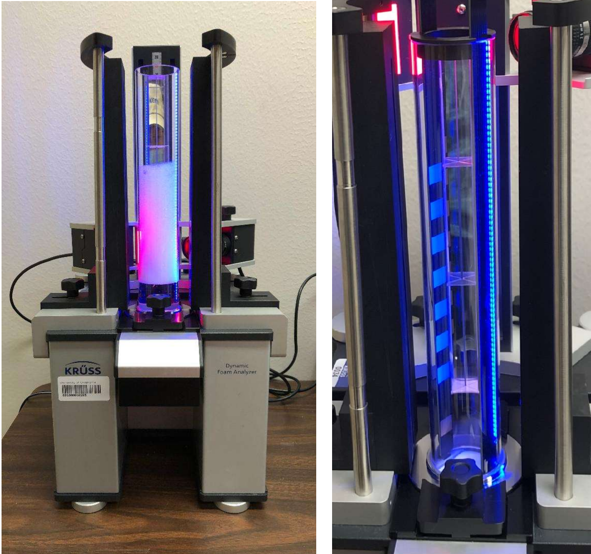
Figure 3.1. Frontal view of the Dynamic Foam Analyzer 100 (DFA100) (left); Liquid content module with electrodes (right).
