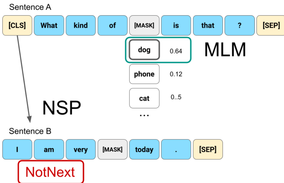
Figure 2.6: The BERT masked language modeling (MLM) and next sentence prediction (NSP) tasks were conducted simultaneously. The MLM task selects the word with the highest predicted probability, which in this case is “dog”. The NSP task predicts whether or not Sentence B directly follows Sentence A, which in this case is false as indicated by the NotNext label. Adapted from (Devlin et al., 2018).
