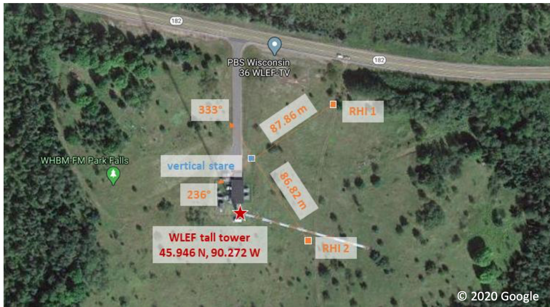
Figure 2.2: A schematic of the lidar deployment strategy at the WLEF tower in Park Falls during CHEESEHEAD. The blue vertical stare lidar was located within SPARC, while the two orange RHI lidars were operated by KIT, constituting a virtual tower. Adapted from Wanner and Mauder (2020).
