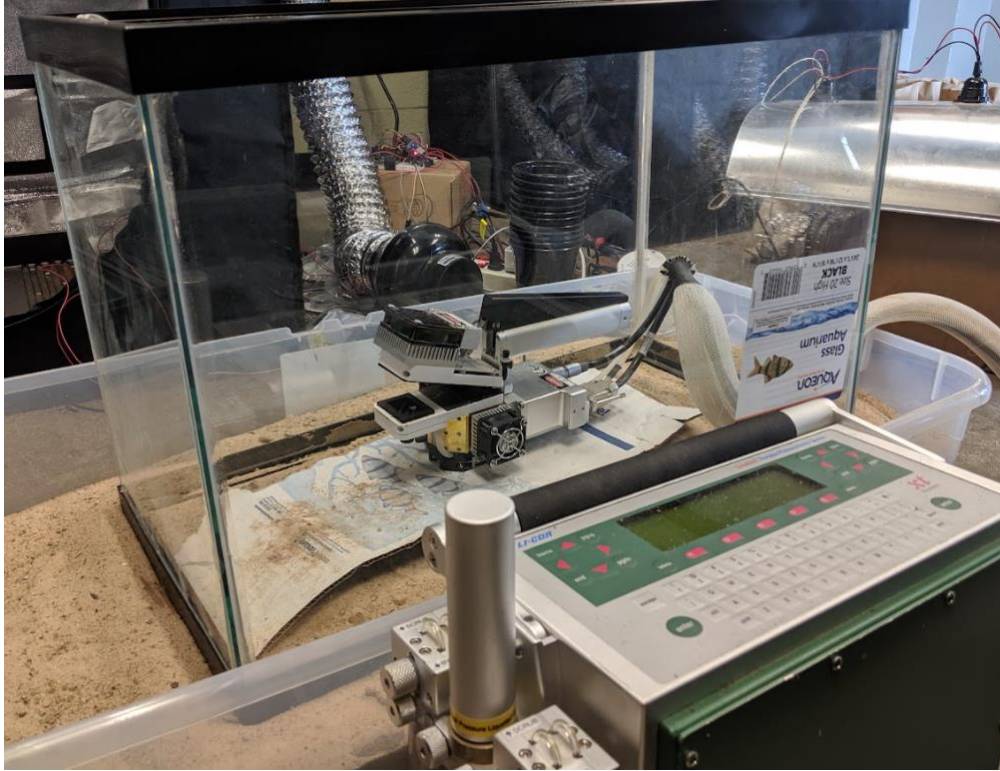
Figure 2: Photograph of whole-plant gas exchange measurement system
