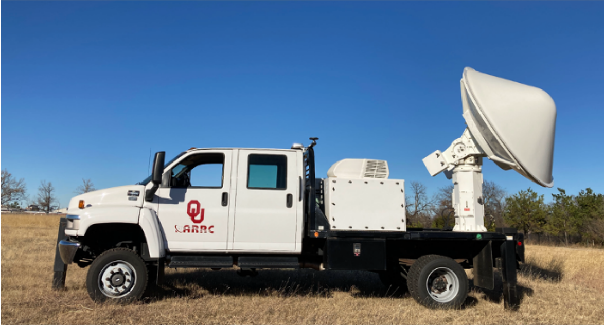
Figure 3.1: An image of the Rapid X-Band Polarimetric Radar (RaXPol) on deployment, courtesy of Dr. David Bodine
