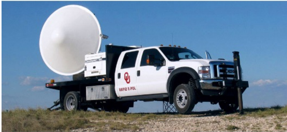
Figure 3.1: Image of the Rapid X-Band Polarimetric Radar (RaXPoI) at the University of Oklahoma
