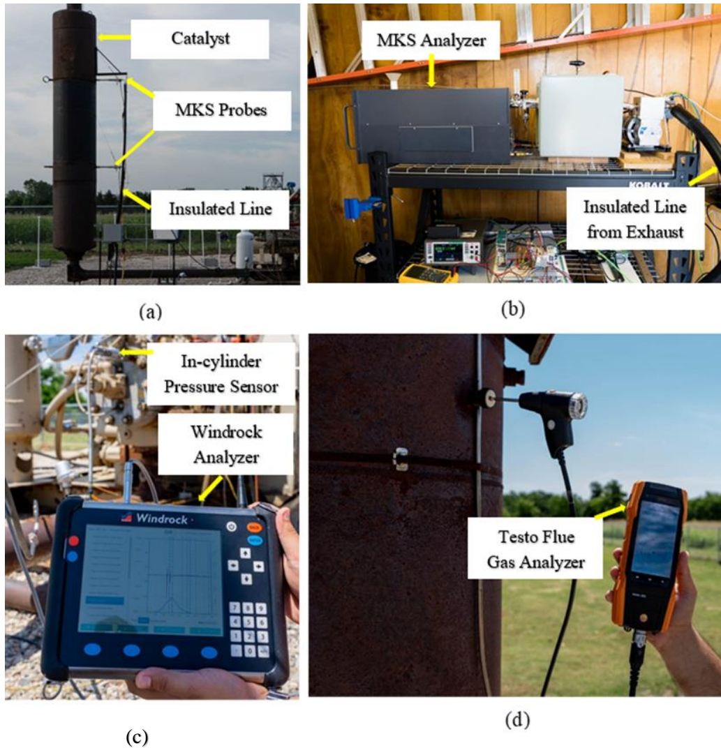
Figure 7. (a) MKS probes on the catalyst. (b) MKS Analyzer inside the Lab. (c) Windrock Portable Analyzer. (d) Testo Flue Gas Analyzer
