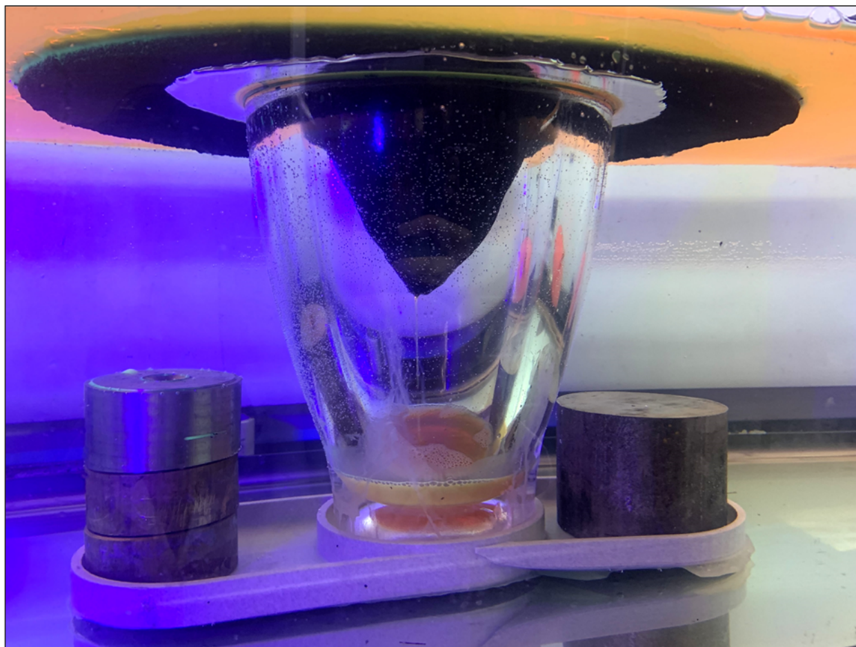
Figure S10. Image of the nanocomposite sponge funnel demonstrating the gravity-driven oil/water separation capabilities in a simulated gasoline spill in water.
