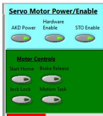
Figure 4-12: Starting motor driver in LabView
