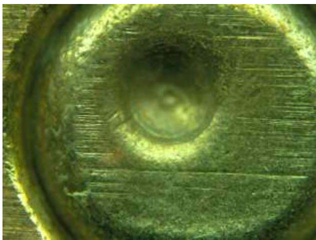
Figure 4: Firing pin impression oriented in the upper/top portion of picture. This orientation was used for all cartridge casings in research.
