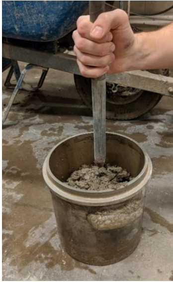
Figure 1.2 shows consolidation of unit weight bowl with internal vibration.
