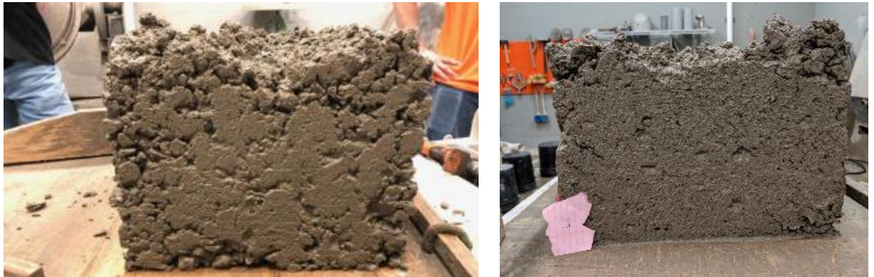
Figure 2.5 Box test results for undesirable mixture (left) and desirable mixture (right)
