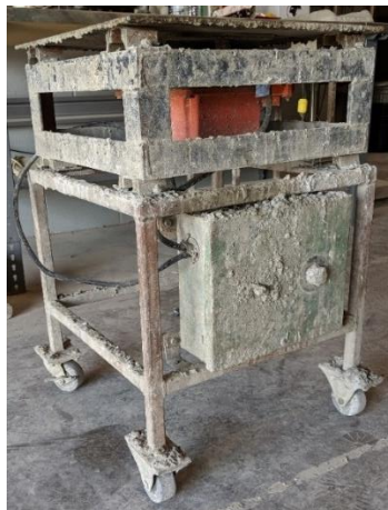
Figure 1.3 displays a typical vibration table powered by a rotary motor.
