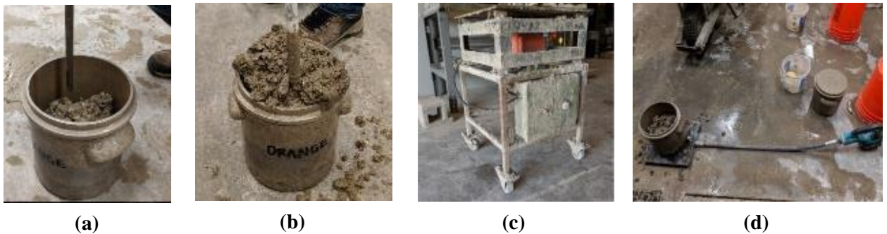
Figure 2.3. (a) rodding, (b) internal vibration with poker vibrator, (c) vibrating table, and (d) MinT
